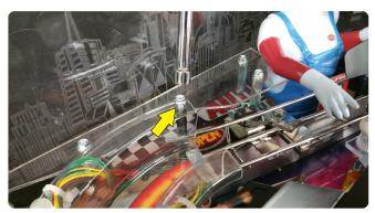
Reinstall 1/4" Screw at top of plastic ramp assembly.
