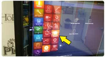
With game powered on, go into Test mode, select Device Tests -> Moving Target.
