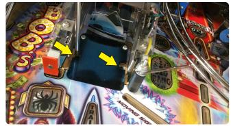
Remove two black screws from bottom of ramp assembly.
