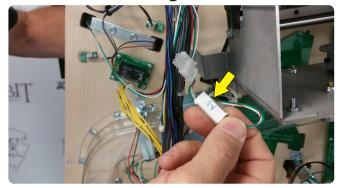
Lift playfield. Unplug the Left Ramp Enter Switch, located near front of plastic ramp assembly.
