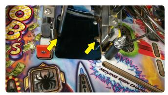
Reinstall both black screws into existing holes at front of ramp assembly.
