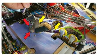
Remove both scoop entrance posts via 1/4" Deep Socket. Then remove Snubber Bracket as indicated.
