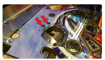
Install front AND back protectors, reinstall Snubber Bracket onto indicated holes.
