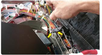
Reposition plastic ramp, align bracket holes with wireform ramp.
