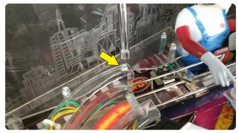
Remove 1/4" Screw from top of ramp assembly.
