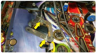
Reinstall both posts, push forward on protector to line up holes.
