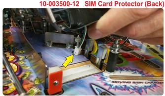
Bring switch plug through hole near front of plastic ramp.
